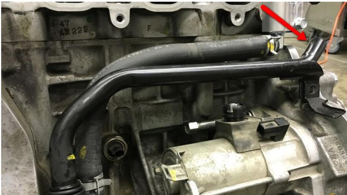
Then use a  $\frac{5}{8}$ " hose coming off this pipe to run to the heater core. The other line comes from the 90 degree  $\frac{1}{2}$ " NPT fitting supplied with the KMiata upper water neck.
