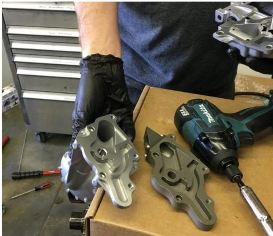
The new chain, new pump, and front pulley all have to go on together. Important: Make sure that the pump is seating completely flush with the bottom of the block. The pump should be
