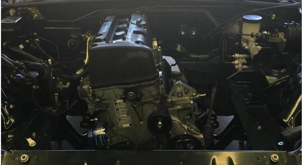
Once this is done, the starter and alternator can be installed in the same manner as any K series engine. Also, the Miata slave cylinder can be bolted back in place, ideally with a braided steel line available from 949 Racing or other companies. If this is done, be sure to bleed the clutch system.
