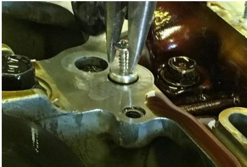
Once it's out, the block will have threads. Simply install a bolt to plug it. Our oil pump kit now includes this bolt, and we like to add some Hondabond on the threads to insure a good seal.
