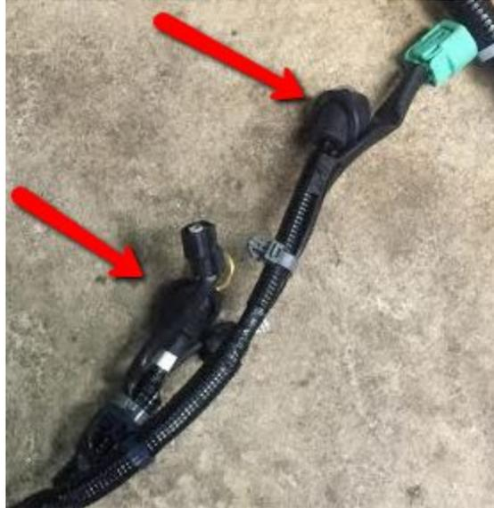
The other smaller connectors go to the alternator and starter as well, and also the knock sensor, like this:
