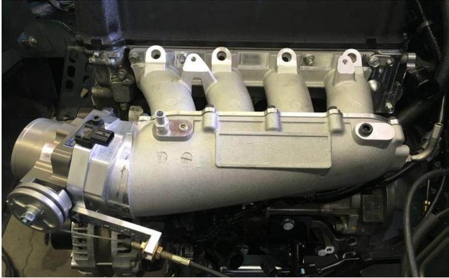
Before installing the throttle body, apply some Hondabond in the B series MAP port on the bottom, since you won't be using it and need to seal it shut.
