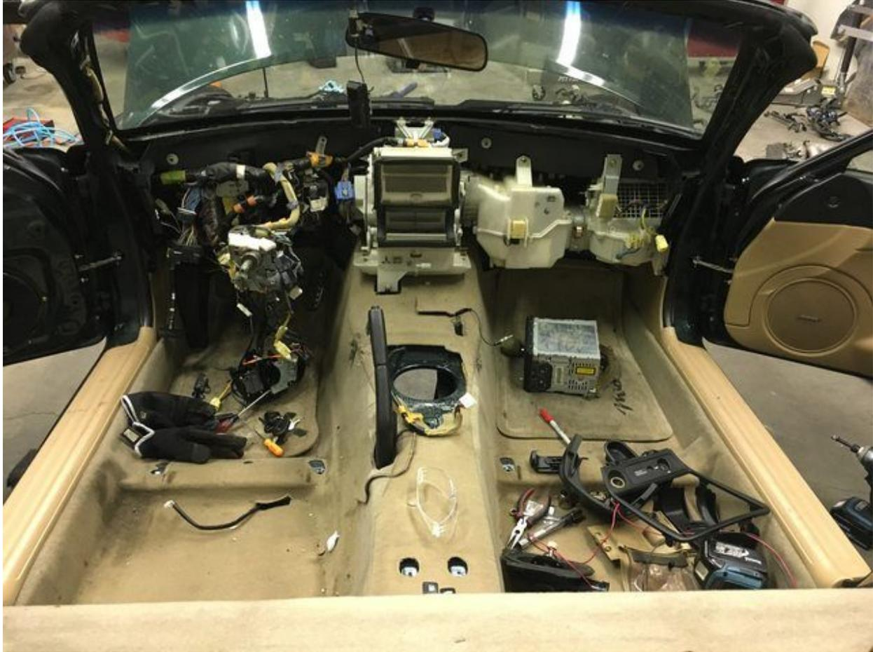
All of the emissions-related components on the passenger side of the vehicle can be removed, as well as the vent line that runs from the charcoal canister back to the fuel tank (some customers may prefer to retain this). The only part that needs to remain is the larger fuel hard line. Please note that an NA Miata will need to retain the return fuel line as well.
