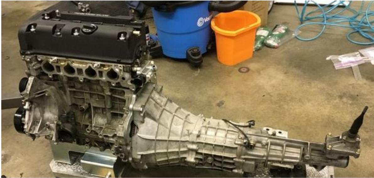
Don't force the transmission input shaft in. with a little finesse, you'll be able to line it up and it should slide right in.
