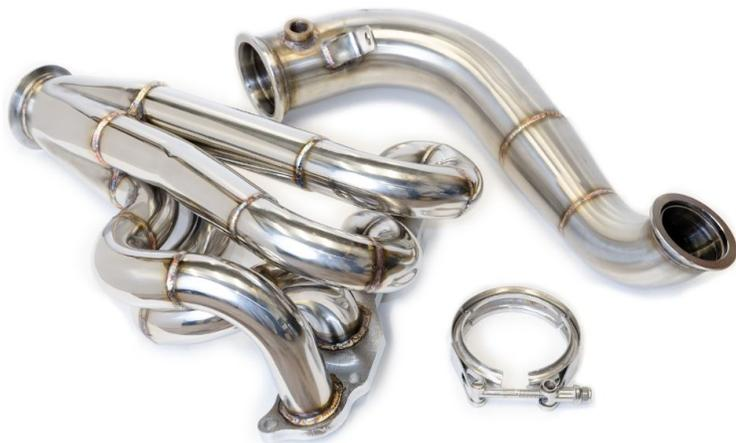
This header includes a mounting tab that bolts behind one of the transmission bolts. This is primarily in place for ease of installation. In road racing and high performance environments, this tab will likely break off. If this is your intended use, please cut the tab before installing the lower section of the header. The rest of your exhaust should be designed so it is supported under the vehicle.
