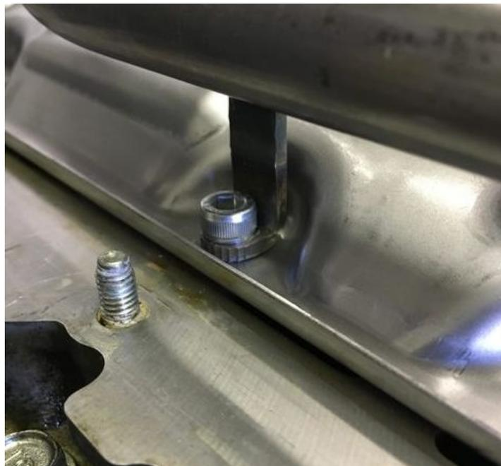
At this point, we have the K20 oil pump with the KMiata adapter, new oil pickup tube, K20 windage tray, and the oil pump chain/tensioners all reassembled and tightened down. Now you can flip the engine back over.
