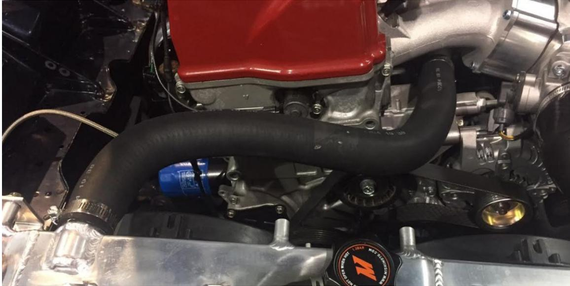
For the lower radiator hose, a universal 135 degree bend pairs well with a K24A2 thermostat housing to point the hose towards the lower radiator inlet.
