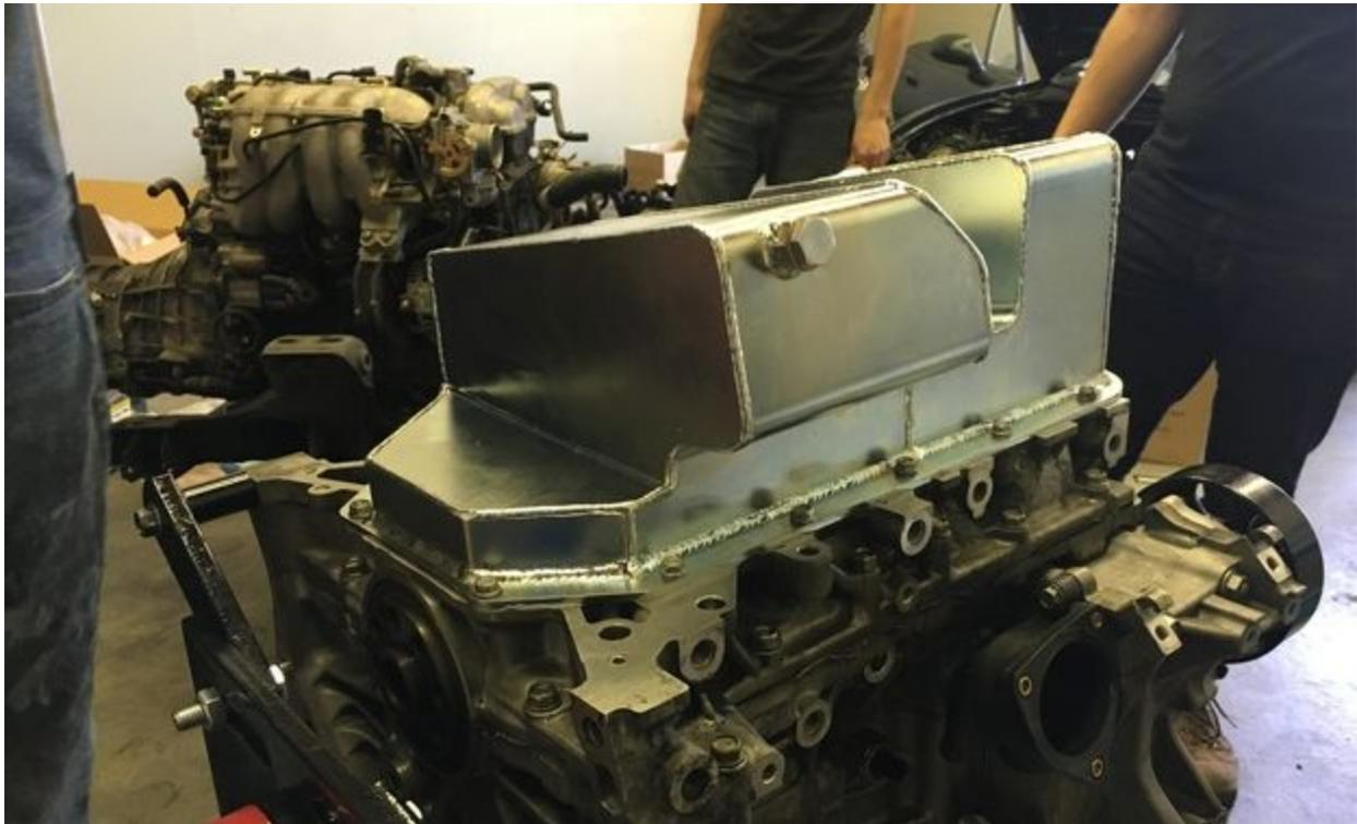
Once everything is dry and tightened up, the engine can be flipped back over, and the timing cover and valve cover can be re-installed.
