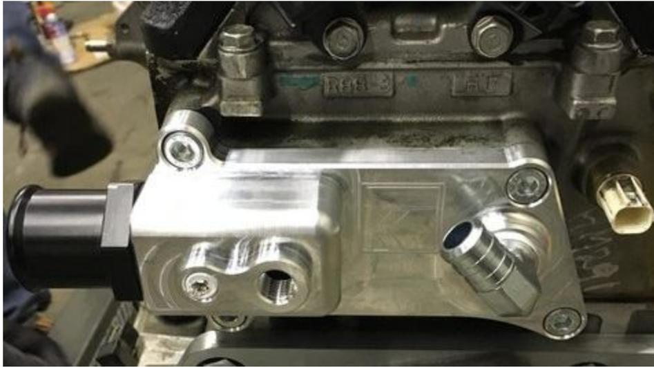
This piece includes three ports, from left to right: 1/8" NPT port for an aftermarket temperature sender, a 12x1.5 port for your OEM Miata temperature sender, and a 1/2" NPT port for a heater hose. Most builds will be configured as shown above, with the 1/8" NPT port plugged, and the 90 degree barbed fitting pointed towards the heater core. Be sure to use teflon tape when installing the NPT fittings.
