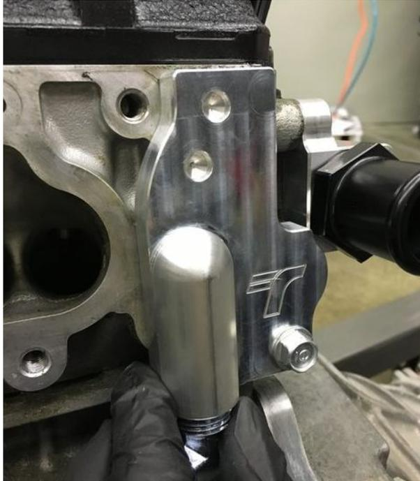
If you plan on retaining heat in the car, you need to cut the black heater pipe out of the thermostat, and add a flexible  $\frac{5}{8}$ " heater hose to the end of it to run to your heater core. The other hose comes out of the KMiata upper water neck piece above.
