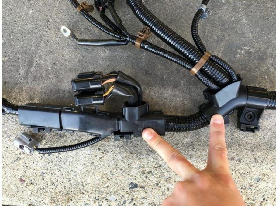
Once this is done, feed the K series harness through the firewall through the same hole as the factory harness, and then begin snapping all the connectors on to the engine. You may want to mock up the intake manifold at this point, but don't tighten it down yet.
