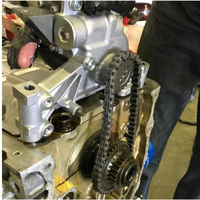
Install the K20 windage tray, but leave it loose. The pickup tube installs on one of the center mounting holes. Use the extra OEM bolt to fasten the pickup tube to the KMiata pump adapter with an o-ring to seal on the pump adapter.
