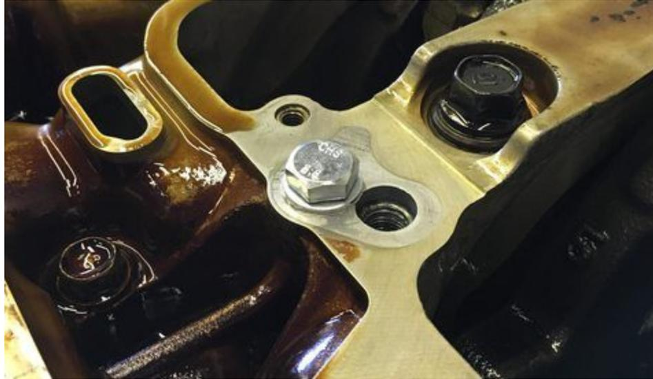
The Type S oil pump will be disassembled and reassembled with a new rear half to adapt to the KMiata pickup tube and oil pan. The factory case half is on the left, with the KMiata part on the right. Just remove the five 10mm bolts and swap the pickup side with the KMiata piece.
