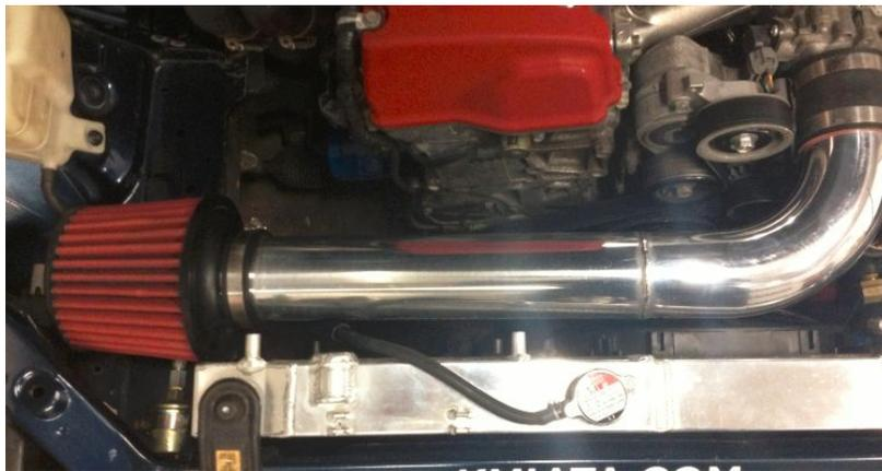
However, for best performance results, keep the intake to the cold side of the engine bay, and ideally run it out of the engine bay altogether for a true cold air intake, like this:
